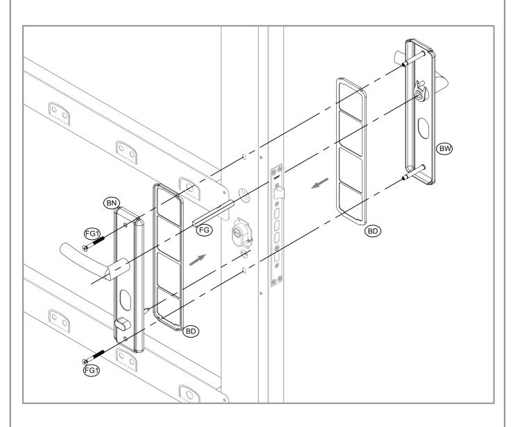
Step 8: Installing the door and lock
