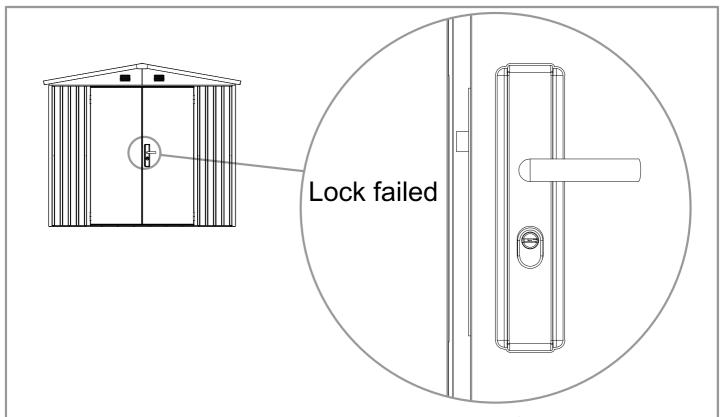
The door gap is too wide and the lock fails. You can use the following methods to adjust.
