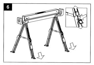
7.Pls loosen the knob and adjust the bracket to the required width and tighten the knob. The range is from 37mm to 90mm to fit different size of plank.
