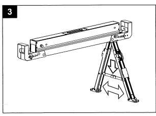
4. Above location labeled "Close 1", press release button and fold down legs until 2x4 supports are fully deployed.
