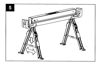
6. Legs adjust in increments of 1 inch. To extend, pull legs down until latch is locked at desired position. To retract, press lock button, pull legs down slightly then push leg up.
