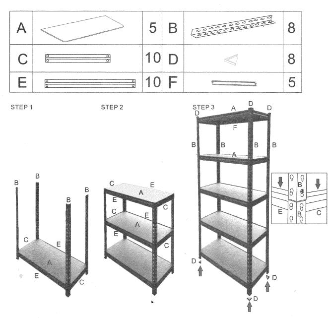
If the tongue is bent, place a screwdriver in the groove and bend in the opposite direction. The whole of the nominal load bearing capacity must not be loaded at one single point on the rack. The load on the inlaid shelves must be evenly distributed in order to avoid damage to the wooden chipboard. The rack is not suitable for rooms with high humidity as this may damage the wooden chipboard.
