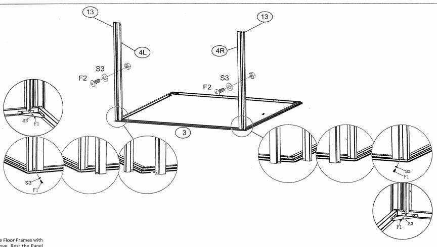
Wall panels ALWAYS attach to the Floor Frames with Screws in the manner shown above .Rest the Panel on the Floor Frame and the holes in the Panel should line up with the holes in the Frame
